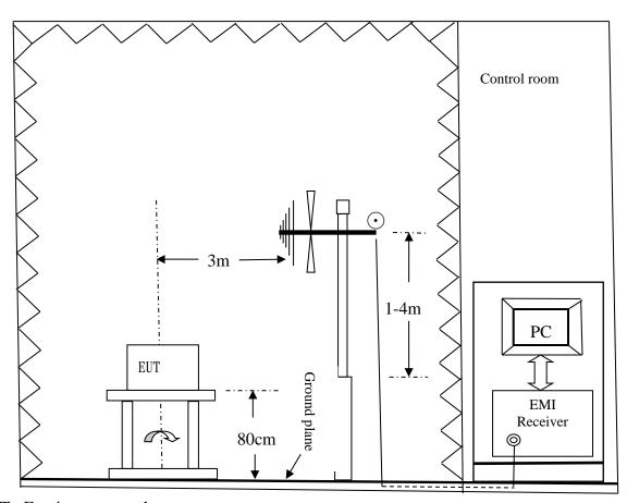
EUT: Equipment under test.
