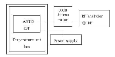
EUT: Equipment under test.
